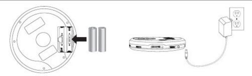
This CD player operates on two 1.5V DC "AA" size (UM-3) alkaline batteries (Not Included) or AC-DC adaptor with an output of 4.5V DC 700mA (Not Included).
