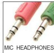
ENLARGED VIEW OF STEREO PLUGS:
