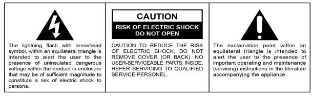
The Caution Marking is located at the bottom enclosure of the apparatus. The Rating plate is located at the bottom enclosure of the apparatus.
