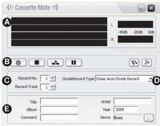
**A. Audio Wave:** If two green bars are present, the JSCR-50 is connected correctly. If green bars are moving and showing a wave pattern, playback is being detected.
